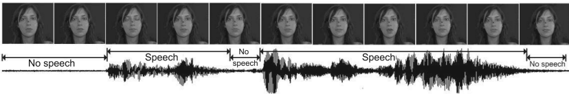
Fig. 11.8. Silence/non-silence detection using multimodal data. Sample taken from eINTERFACE 2005 database: “Oh my god, there is someone in the house!”.
