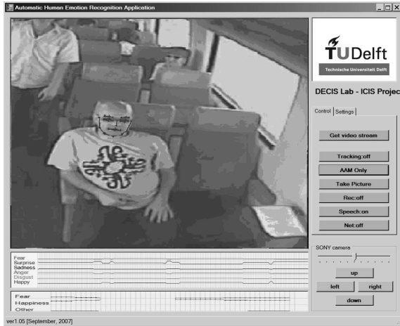
Fig. 11.16. A snapshot during a working session; experimental setup with our software implementation of the emotion recognition system.
